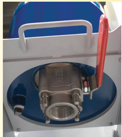
Bottom of tank showing ball valve and plug for draining water jacket.
