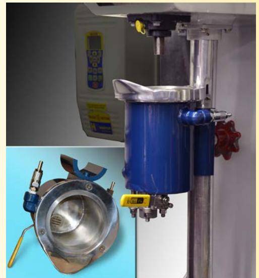
One-piece tank showing bottom discharge grid and valve.
