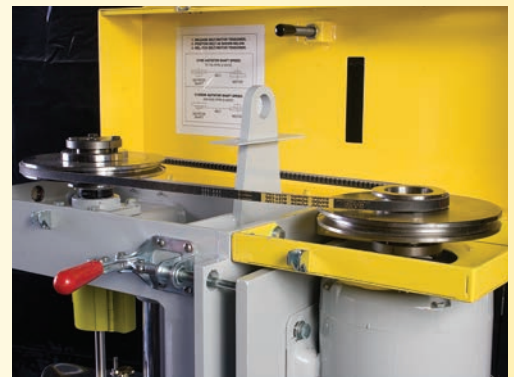
Belt guard raised to show pulleys for quick change-over from Model HDDM-01 to HD-01 mode.
