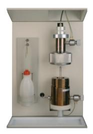
porosity approaching the micropore region. Thanks to its high pressurization speed, it is highly recommended in QC labs where short run times and productivity are the priorities.
