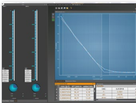
CMC determination with DCATS 33
